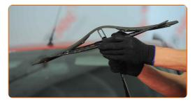
Remove the blade from the wiper arm.
