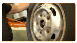
Unscrew the axle nut. Use a 36 mm socket. Use a ratchet wrench.
