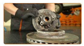
Clean the brake disc surface that is in contact with the wheel rim. Use a wire brush.
