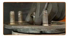
Detach the brake disc from the wheel hub.
