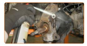
Clean the splines of the CV joint. Use a wire brush. Use an all-purpose cleaning spray.
