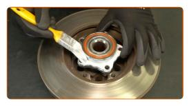
Install the wheel hub together with brake disc.
