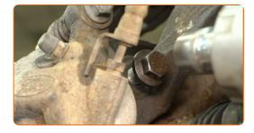
Tighten the fasteners of the brake caliper bracket. Use an 18 mm socket. Use a torque wrench. Tightening torque: 175 N·m.
