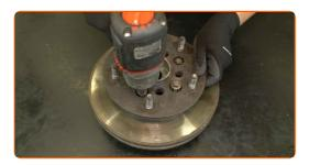
Treat the mounting surface on the wheel bearing. Use ceramic grease.
