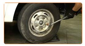
Tighten the axle nut. Use a 36 mm socket. Use a torque wrench. Tightening torque: 320 N·m.
