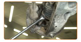
Remove the fastening bolts. Use a ratchet wrench.
