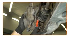
Unscrew the brake caliper bracket fasteners. Use an 18 mm socket. Use a tommy bar.
