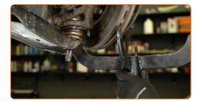
Disconnect the ball joint from the control arm. Use a ball joint separator.
