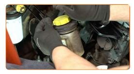
Release the clamp of the lower coolant hose. Use hose clamp pliers.
