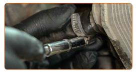
Screw in the coolant drain plug.
