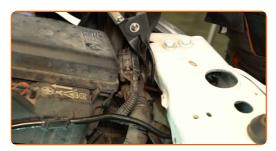
Detach the power steering fluid reservoir.
