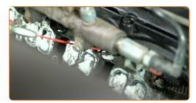
Unscrew the glow plugs. Use a 10 mm glow plug socket. Use a torque wrench.
