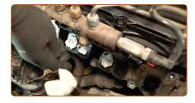
Unscrew the nuts that connect the power terminals to the glow plugs. Use a 7 mm socket. Use a ratchet wrench.
