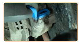
Unscrew the lower fasteners of the engine mount. Use a 13 mm socket. Use a ratchet wrench.
