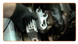
11 Install the fastening nuts and bolts.
