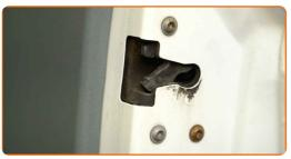
Unscrew the fastener of the exterior door handle. Use a 10 mm socket. Use a ratchet wrench.
