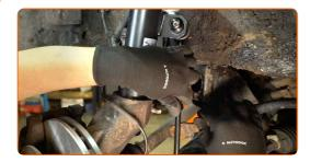
Tighten the fastener connecting the anti-roll bar link to the anti-roll bar. Use a 20 mm combination spanner. Use a 17 mm socket. Use a torque wrench. Tightening torque: 55 N·m.
