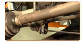
Unscrew the fastener connecting the anti-roll bar link to the suspension strut. Use a 19 mm socket. Use a ratchet wrench.
