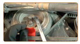
Remove the alternator V-ribbed belt by turning the crankshaft pulley. Use a stretch belt removal/fitting tool. Use a mounting lever. Use a 15 mm combination spanner.
