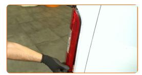
Tighten the fasteners connecting the rear light to the car body.
