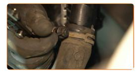
Install the power steering fluid reservoir on the upper radiator support cover.
