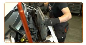
Remove the lower insulators of the radiator.
