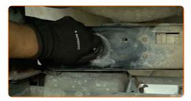
Remove the engine cooling fan shroud together with the fan from the radiator. Use a mounting lever.
