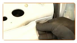
Unscrew the fasteners of the upper radiator support cover. Use a 13 mm combination spanner. Use a 13 mm socket. Use a ratchet wrench.
