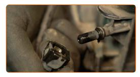
Detach the overflow hose from its brackets on the radiator.
