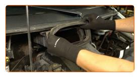
Install a new filter into the housing. Check the markings on the edge of the filter to make sure you are installing it the correct side up.
