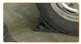
Loosen the wheel nuts. Use a 21 mm wheel impact socket. Use a tommy bar.
