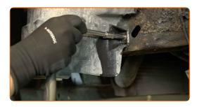
10 Remove the fastening bolt.
