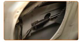
Install the fastening bolt of the window guide rail.
