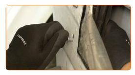
Unscrew the fasteners of the window regulator mechanism. Use a 10 mm socket. Use a ratchet wrench.
