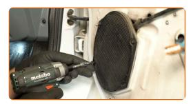
Remove the fastening screws.
