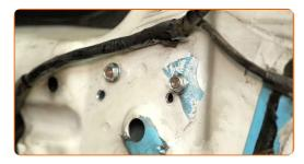
Tighten the fasteners of the window regulator mechanism. Use a 10 mm socket. Use a torque wrench. Tightening torque: 8 N·m.
