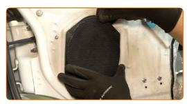
Install and screw in the fastening screws of the speaker. Use a Phillips screwdriver.
