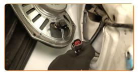
Detach the connector from the power window motor.
