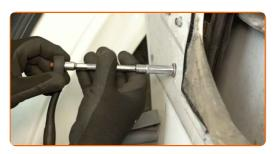
Remove the fastening bolt.
