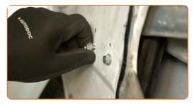
Remove the window regulator mechanism.
