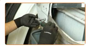
Install the rivets connecting the glass to the window regulator mechanism. Use a riveter. Use rivets.
