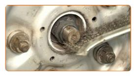
Loosen the axle nut. Use a 36 mm socket. Use a tommy bar.
