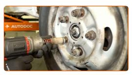
Lower the car and tighten the wheel nuts in a criss-cross order. Use a 21 mm wheel impact socket. Use a torque wrench. Tightening torque: 200 N·m.
