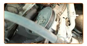
Fit a new alternator V-ribbed belt by turning the crankshaft pulley. Use a stretch belt removal/fitting tool. Use a 15 mm combination spanner.
