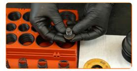
17 Install a new O-ring on the oil filter cap.
