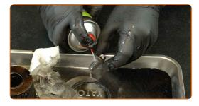
16 Install a new O-ring on the drain plug.
