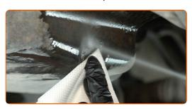
Screw in the drain plug and tighten it. Use a 13 mm socket. Use a torque wrench. Tightening torque: 23 N·m.
