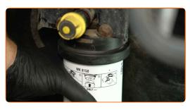
Replacement: fuel filter – FORD Transit Mk6 Minibus (V347, V348). Tip from AUTODOC:
