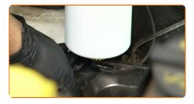
Remove the fluid drain pan from under the fuel filter.
