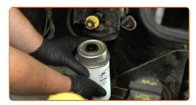
Install the new filter and secure it in its mounting seat.
