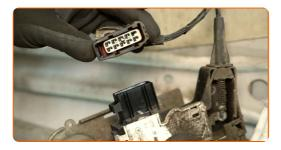
Detach the door latch cable from the lock.
