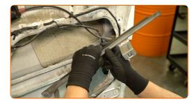
Unscrew the door lock fasteners. Use a T30 Torx bit. Use an electric or ratchet screwdriver.
