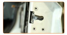
20 Install the fastening screws.
