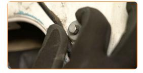
Tighten the window guide rail fasteners. Use an 8 mm socket. Use a torque wrench. Tightening torque: 10 N·m.
