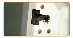
Unscrew the fastener of the exterior door handle. Use a 10 mm socket. Use a ratchet wrench.
