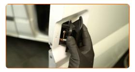
Tighten the door handle fastener. Use a 10 mm socket. Use a torque wrench. Tightening torque: 10 N·m.
