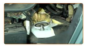
Clean the fasteners of the top strut mount. Use a wire brush. Use WD-40 spray.
