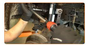
Tighten the fastener of the ABS sensor cable bracket. Use an 18 mm socket. Use a torque wrench. Tightening torque: 45 N·m.
