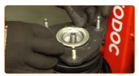
Install and tighten the strut piston rod nut. Use an 18 mm strut nut socket. Use an H6 hex extension bar. Use a torque wrench. Tightening torque: 70 N·m.
