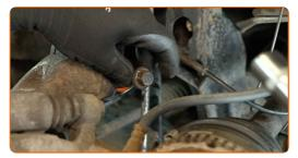
Disconnect the steering knuckle from the suspension strut. Use a rubber mallet. Use a transmission jack or one more vehicle jack.
