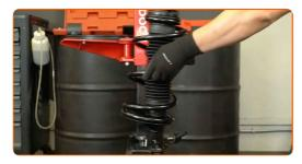
Install the strut assembly into the wheel arch.
