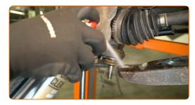
Attach the ball joint to the suspension arm and screw on the fastening nut. Use a mounting lever.
