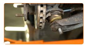
Install the anti-roll bar link and screw on the fastening nut.
