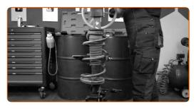
Remove the mount bearing and the bump stop.
