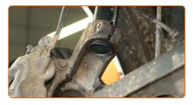
Install and screw in the fastening bolt.
