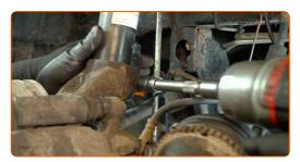
Remove the fastening bolt.
