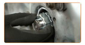
Install the cotter pin. Use a mounting lever.
