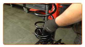
Install a dust boot, bump stop, and mount bearing.
