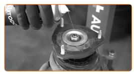
Unscrew the strut piston rod nut. Use an 18 mm strut nut socket. Use an H6 hex extension bar. Use a ratchet wrench.
