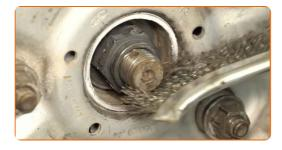
Loosen the axle nut. Use a 36 mm socket. Use a tommy bar.
