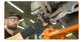
Disconnect the ball joint from the suspension arm. Use a ball joint separator. Use a mounting lever.
