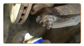
Unscrew the fastener connecting the ball joint to the suspension arm. Use a 24 mm socket. Use a ratchet wrench.
