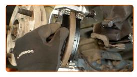
Attach the wear sensor to the inner pad.
