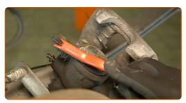
17 Retract the brake caliper piston. Use a brake caliper wind back tool.
