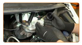
Tighten the brake fluid reservoir cap.
