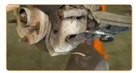
10 Unscrew the brake caliper fasteners. Use a 21 mm combination spanner.
