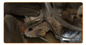
14 Remove the brake pads.
