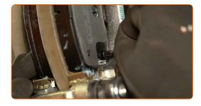
21 Install the brake caliper.
