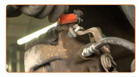
9 Spread the brake pads apart. Use a mounting lever.
