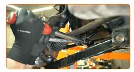
Clean the mounting seat of one of the wheels. Use a wire brush. Use an all-purpose cleaning spray.
