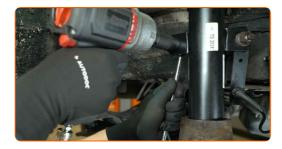
Remove the anti-roll bar link.
