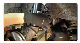
Tighten the fastener connecting the anti-roll bar link to the anti-roll bar. Use a 20 mm combination spanner. Use a 17 mm socket. Use a torque wrench. Tightening torque: 55 N·m.
