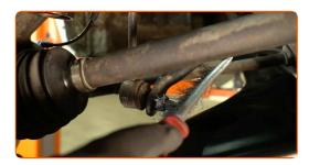
Unscrew the fastener connecting the anti-roll bar link to the anti-roll bar. Use a 19 mm combination spanner. Use an H5 Allen key to secure the ball stud. Use a ratchet wrench.
