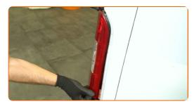
Tighten the fasteners connecting the rear light to the car body.
