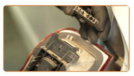
Remove the bulb holder together with the bulbs.
