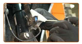
Attach the connector of the brake pad wear sensor.
