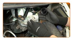
Tighten the brake fluid reservoir cap.
