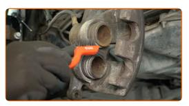
Retract the brake caliper pistons. Use a brake caliper wind back tool.
