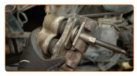
Treat the brake pads in the areas where they contact the brake caliper bracket. Use anti-squeal paste.
