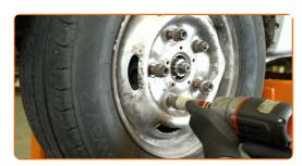
Lower the car and tighten the wheel nuts in a criss-cross order. Use a 21 mm wheel impact socket. Use a torque wrench. Tightening torque: 200 N·m.
