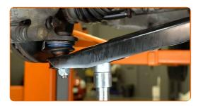
Tighten the front fastener of the control arm. Use a 21 mm combination spanner. Use an 18 mm socket. Use a torque wrench. Tightening torque: 200 N·m.
