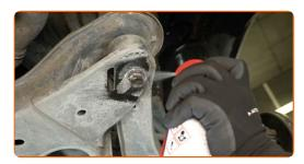
Unscrew the fastener connecting the ball joint to the control arm. Use a 24 mm socket. Use a ratchet wrench.
