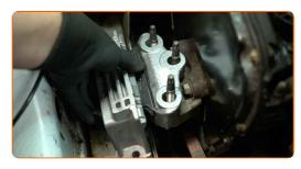
11 Install the fastening nuts and bolts.
