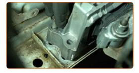
Tighten the upper fasteners of the engine mount. Use an 18 mm socket. Use a torque wrench. Tightening torque: 115 N·m.
