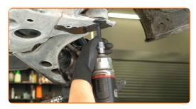
Remove the fastening bolt.
