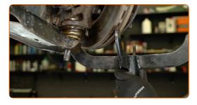
Disconnect the ball joint from the control arm. Use a ball joint separator.
