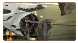
Unscrew the front fastener of the control arm. Use a 21 mm combination spanner. Use an 18 mm socket. Use a ratchet wrench.
