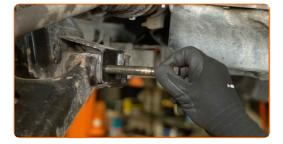
Remove the control arm. Use a mounting lever.
