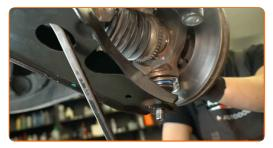
Tighten the fastener that connects the control arm to the ball joint. Use a 24 mm socket. Use a torque wrench. Tightening torque: 150 N·m.
