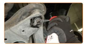
Unscrew the fastener connecting the ball joint to the control arm. Use a 24 mm socket. Use a ratchet wrench.
