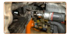
Remove the fastening bolt.
