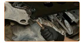
Attach the ball joint to the control arm by screwing on the nut.
