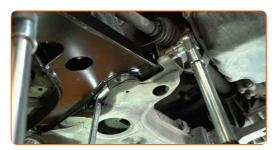
Clean the wheel rim mounting seat. Use a wire brush. Use an all-purpose cleaning spray.
