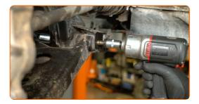
14 Remove the fastening bolt.
