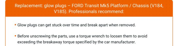
• If you have reached the breakaway torque but the glow plugs still will not loosen up, you need to seek professional help: a glow plug fragment left inside the well or damage to the thread of the mounting seat can result in costly engine repairs.
