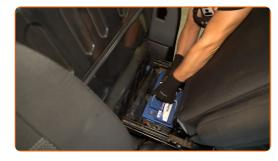
Connect the positive terminal to the battery.
