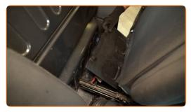
Unscrew the negative battery terminal fastener. Use a 10 mm socket. Use a ratchet wrench.
