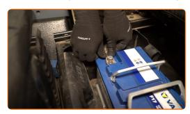
Screw in the negative battery terminal fastener. Use a 10 mm socket. Use a ratchet wrench.
