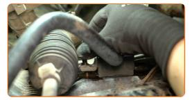
Remove the anti-roll bar bush bracket.
