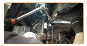
Tighten the fastener connecting the anti-roll bar link to the suspension strut. Use a 20 mm combination spanner. Use a 17 mm socket. Use a torque wrench. Tightening torque: 55 N·m.
