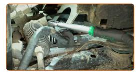
Clean the mounting seats of the anti-roll bar link on one side of the axle. Use a wire brush. Use an all-purpose cleaning spray.
