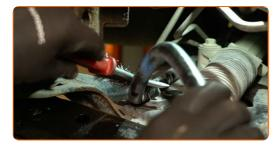
Install a new anti-roll bar bush on one side of the axle.
