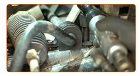
Tighten the fasteners on both anti-roll bar bush brackets. Use a 10 mm socket. Use a torque wrench. Tightening torque: 25 N·m.
