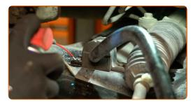
Clean the mounting seats of the anti-roll bar bushes. Use a wire brush. Use an all-purpose cleaning spray.
