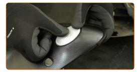
Reattach the connector to the turn signal repeater light.
