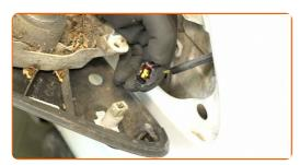
Treat the connector of the turn signal repeater light. Use an electronic spray.
