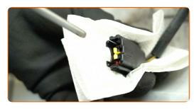
Remove the turn signal repeater light.
