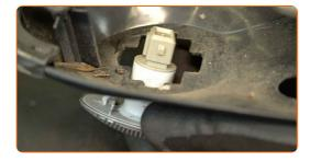
Install the turn signal repeater light on a new wing mirror.
