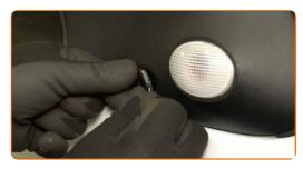
Unscrew the wing mirror fasteners. Use an 8 mm socket. Use a ratchet wrench.
