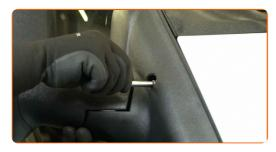
Screw in the wing mirror fasteners. Use an 8 mm socket. Use a ratchet wrench.
