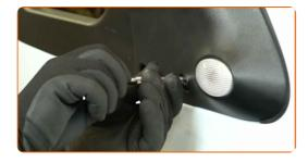
Install the covers of the wing mirror fasteners.
