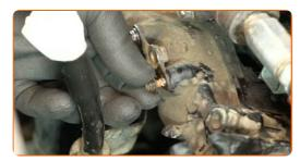
Clean the intake manifold fasteners. Use a wire brush. Use WD-40 spray.
