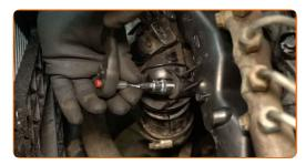
Install the fasteners of the oil dipstick tube bracket.
