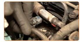
Detach the wiring harness fastener and move the harness aside. Use a clip removal tool.
