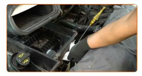
Plug the oil dipstick hole with a paper towel to prevent dirt from entering the system.
