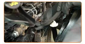
Attach the camshaft position sensor connector.
