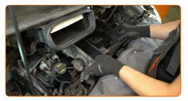
Clean the connectors of the fuel pressure, MAP and camshaft position sensors. Use an all-purpose cleaning spray.
