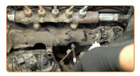
Remove the intake manifold.
