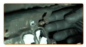
Remove the terminals and move the glow plug wire out of the way.
