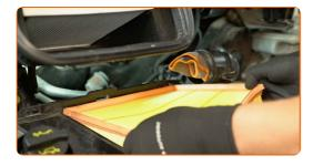
Unscrew the fasteners of the air filter housing. Use a 10 mm socket. Use a ratchet wrench.
