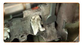
Remove the intake manifold gaskets.
