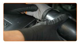
Connect the air intake hose to the air filter housing.
