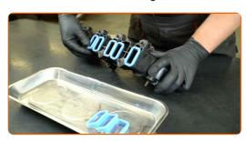
Remove the paper towels from the intake manifold openings.
