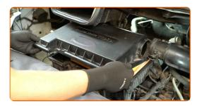
Plug the air intake hose with a microfibre towel to prevent dust and dirt from getting into the system.
