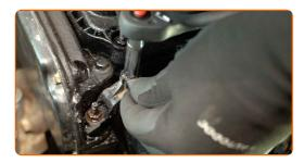
Detach the fuel pressure sensor connector.
