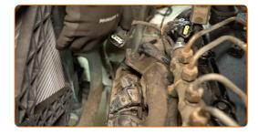
Detach the camshaft position sensor connector.
