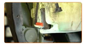
Remove the windscreen washer pump. Use hose removal pliers.
