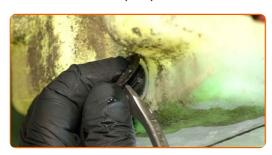
Clean the mounting seat of the windscreen washer pump. Use an all-purpose cleaning spray.
