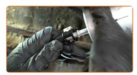
Screw in the fuel filter mounting bracket. Use a drive socket #8. Use a ratchet wrench.
