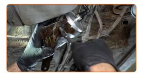
Screw in the fastening bolts of the fuel filter bracket. Use a drive socket #10. Use a ratchet wrench.
