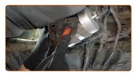
Unscrew the fuel filter bracket. Use a drive socket #8. Use a ratchet wrench.
