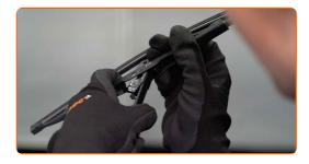
Remove the blade from the wiper arm.
