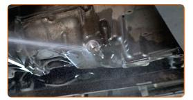
18 Screw in the new drainage plug and tighten it. Use a drive socket #21. Use a torque wrench. Tighten it to 26 nm torque.
