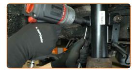
Remove the anti-roll bar link.
