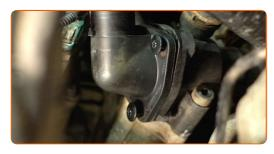
Tighten the fasteners of the thermostat housing cover. Use a T30 Torx bit. Use a U-joint socket extension. Use a torque wrench. Tightening torque: 10 N·m.
