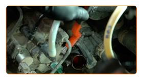
Unscrew the fasteners of the thermostat housing cover. Use a T25 Torx bit. Use a U-joint socket extension. Use a ratchet wrench.
