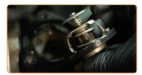
Clean the mounting seat of the thermostat housing cover. Use an all-purpose cleaning spray.
