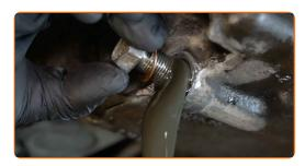
Replacement: engine oil and filter – FORD Transit Custom V362 Minibus (F3).
