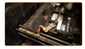
Remove the positive terminal from the battery.
