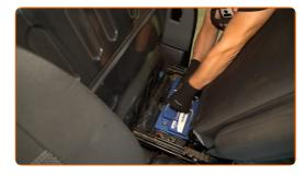
Connect the positive terminal to the battery.
