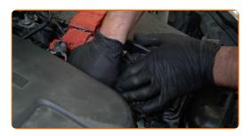
Remove the air filter housing.
