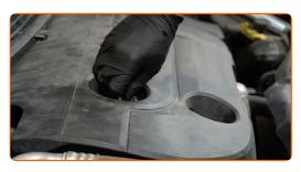
Tighten the oil filler cap.
