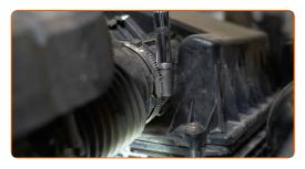
11 Remove the air intake pipe. Use a crowbar.
