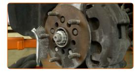
Treat the wheel hub surface that contacts the wheel rim. Use ceramic grease.
