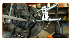
Unscrew the tie rod end from the tie rod.
