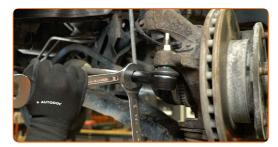
Tighten the nut connecting the tie rod end to the steering knuckle. Use a 19 mm socket. Use a torque wrench. Tightening torque: 80 N·m.
