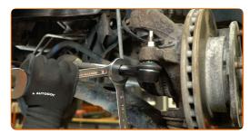
Tighten the nut connecting the tie rod end to the steering knuckle. Use a 19 mm socket. Use a torque wrench. Tightening torque: 80 N·m.
