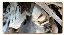
Tighten the fasteners of the oil pan lower cover. Use Torx T30. Use a ratchet wrench.
