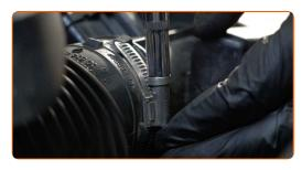
Connect the crankcase ventilation hose to the air duct.
