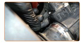
Plug in the mass air flow sensor conntector.
